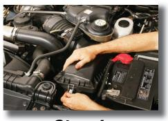
Step 4: Reconnect wiring harnessess to the MAFS sensor, filter minder, the coolant reservoir and positive battery cable. You're Done!
