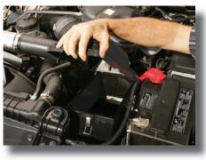
Step 2: The conversion housing fits into the OEM footprint. To install, press the pins on the housing's bottom in the battery tray grommets.
