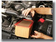
Step 3: Place the WIX Powertrap<sup>®</sup> air filter in the housing, locking all tabs and clamps.
